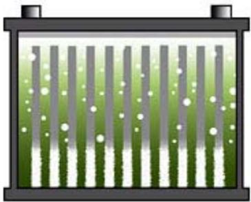
**Figure 2: Stratified battery**
