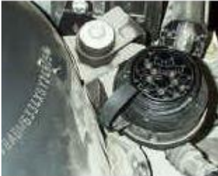
20 Pins DLC located at the Engine compartment
